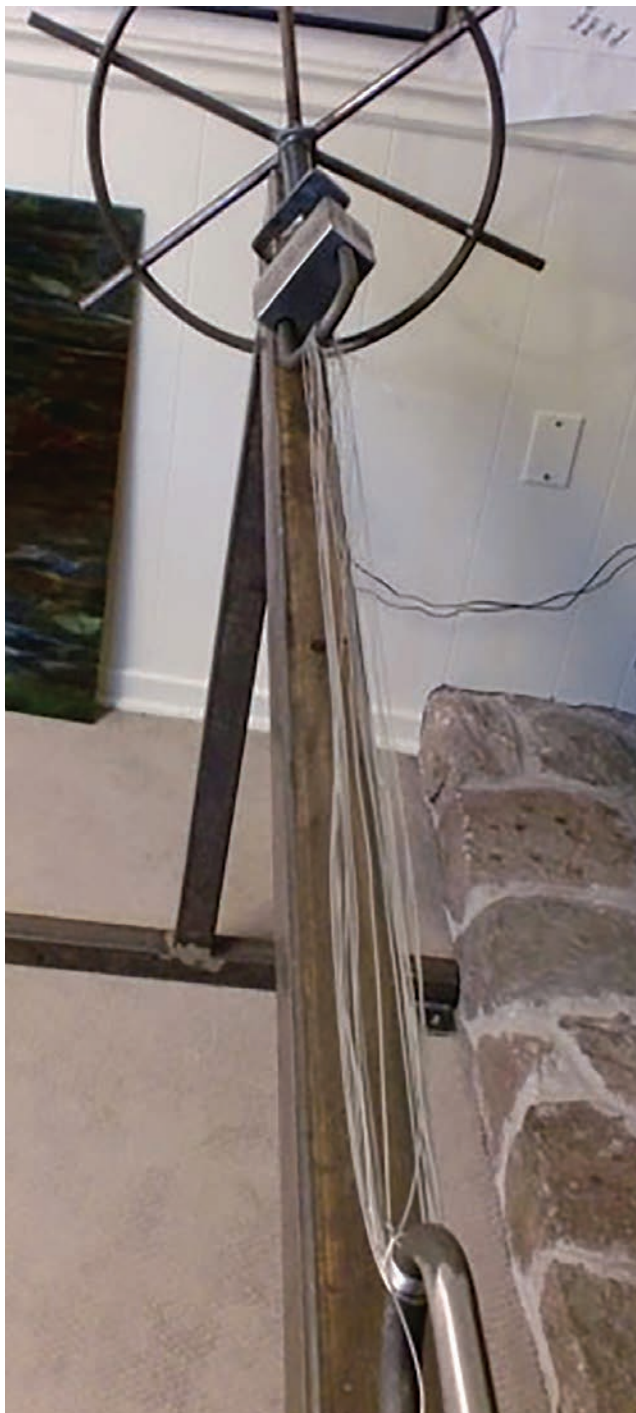
Fig. 3 – Wire spinner fabricated by John MacDonald for Seaton.
